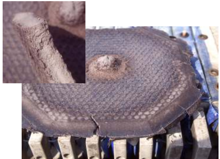
Sludge was dewatered using an IWWS filter press and the resulting filter cake was sent to the lab for analysis. The filter cake was very dry and easily handled.
