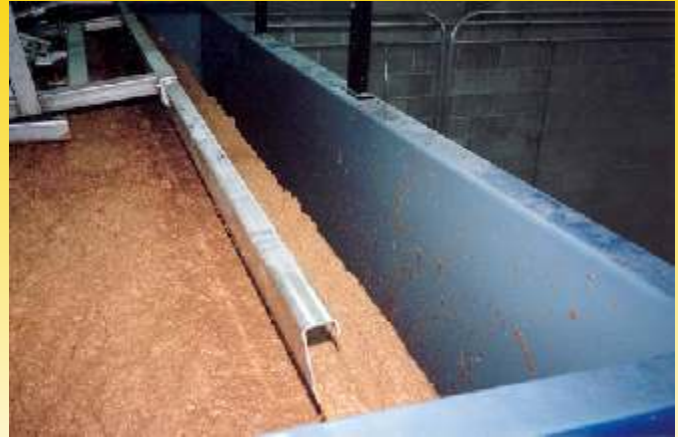
IWWS Physical/Chemical Waste Treatment System showing clean effluent overflow (left), sludge removal (center) and sludge holding compartment (right).
